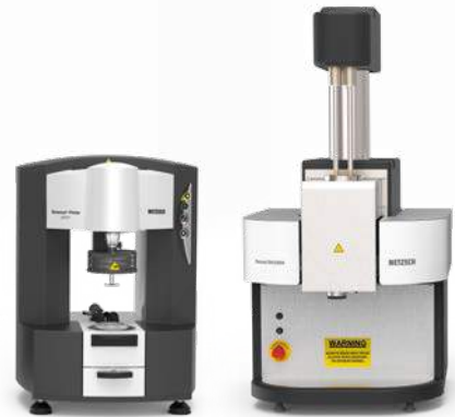
Viscosity measurement of a shower gel at room temperature over a wide shear rate range utilizing both a Rosand capillary rheometer as well as a Kinexus rotational rheometer
