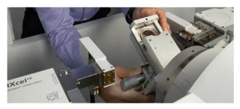
Research programs change and materials projects follow new directions. With PreFIX technology, the X'Pert<sup>3</sup> system can easily be upgraded as new applications arise or when new optics are available. The different optical configurations show no compromise in resolution or intensity when switching between applications.
