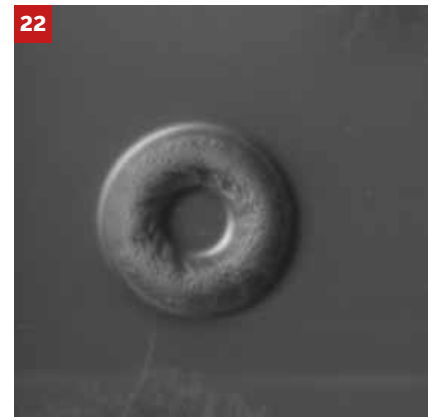
Fig. 22: The Flood Gun effectively compensates for sample charging. FIB milling carried out with no charge compensation.
