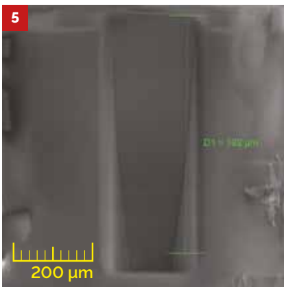
Fig. 5: Milling into a glass layer for reaching the IC board. Probe window: 200 \times 200 \times 592 \mu\text{m}^3 . Milling time with Xe plasma ion at 2 \mu\text{A} : 14 hours. Milling time with Ga LMIS at 65 \text{ nA} : more than 20 days.
