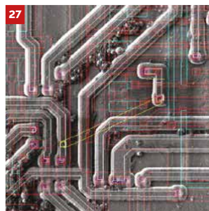
Fig. 27: Design data superimposed on top of FIB image for circuit editing.
